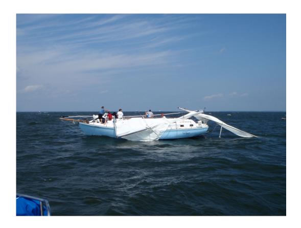
We motored to dock and began further assessments. It turned out that a bronze turnbuckle was the culprit. This turnbuckle gave way on the main shroud and caused the intense destruction. Now I needed a repair plan. After weighing several options including sleeves and patch repairs, I decided on a new mast for "*VelAmore*". The progress on this is well underway but slower than I'd like…but she is going to be ok after all.
