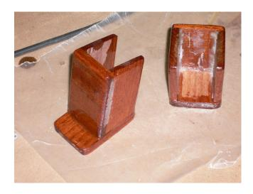
This next picture shows the brackets I made to attach the davits to the stern rail.
